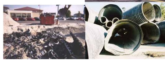
tions, which required using a Class I or Class II backfill material for a fully encapsulated backfill envelope, were not followed. Instead, a Class I stone material was placed up to the springline and in situ material was used for the balance of the backfill. This failure, which occurred early in the project, delayed the work to complete the parking lot and begin construction of the buildings in the office park.
