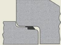
Concrete joints with a groove or offset on the spigot and/or bell utilize a rubber compound gasket, which fits against the shoulder or in the groove of the joint.
