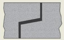
Joints utilizing flexible mastic sealants typically perform as a soil tight system unless higher performance expectations are described in the project specifications.
