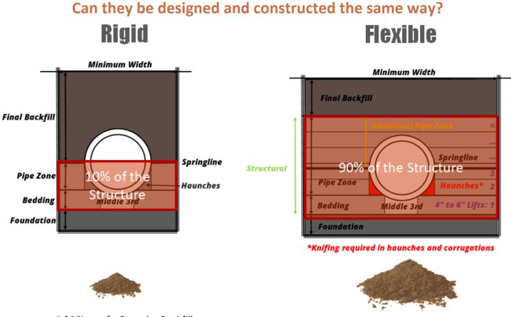
3 ft³/linear ft. Granular Backfill
