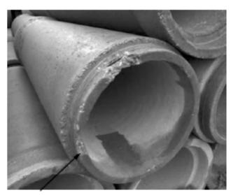
Figure 22—Repairable Chipped End of Spigot (Photo Courtesy of ACPA)
