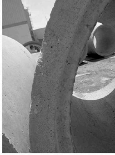
Figure 9—Acceptable Chip on Bell End (Photo Courtesy of ACPA)
