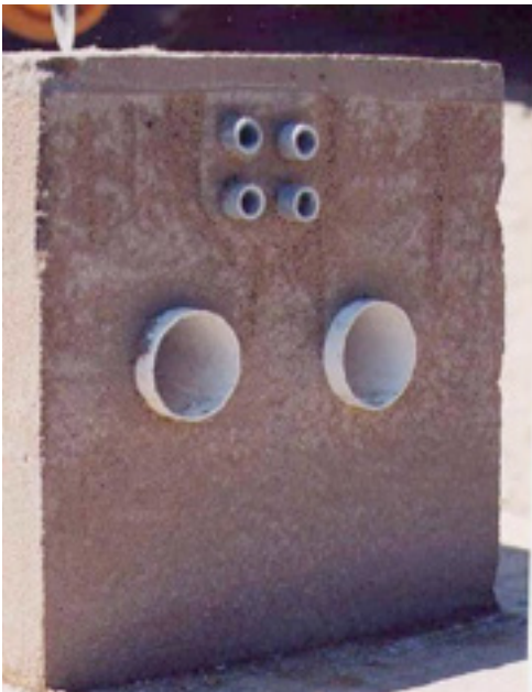
Figure 2. Cured Flowable Fill
