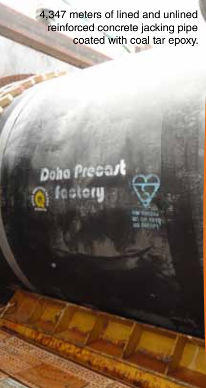
Standard GRP-lined jacking pipe coated with coal tar epoxy for sanitary sewer conveyance system in Bahrain.
