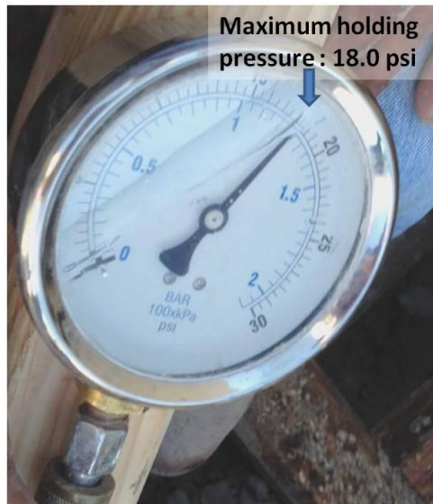
Figure 8 Maximum holding pressure in 24 in. RCP with a mechanical core of 2.78 in
