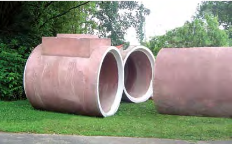
Red dye mixed with additive to verify even distribution through each pipe. Additive provided additional protection against potential of sulfuric acid corrosion.
