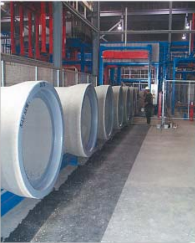
Royal's new Shlusselbauer Exact 2500 production plant produced the 36-inch diameter RCP used for the Wilmes Lake Sanitary Sewer Trunk deep installation project.
