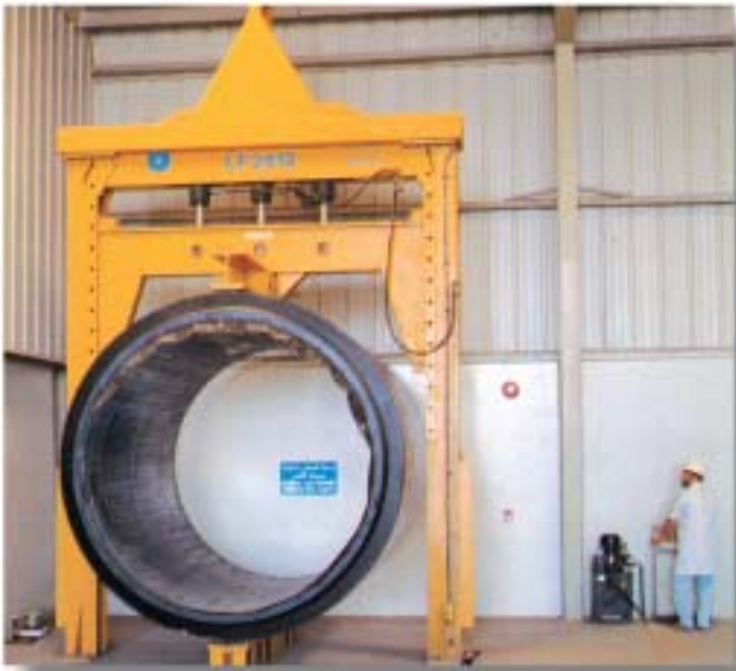
A 2400-mm (96-inch) diameter Class IV reinforced concrete pipe undergoes a three-edge bearing test as part of Advanced Pipes and Cast Company's extensive quality assurance
