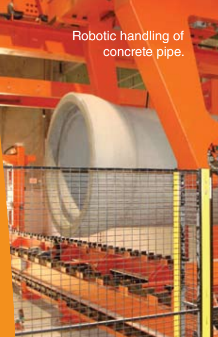
Mass production of small diameter NRCP at The Langley Concrete Group of Companies in Chilliwack, B.C., Canada.
