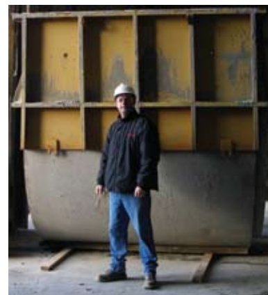
Standard 84-inch diameter RCP prepared for wet cast of pre-bed. Photo Credit: Dennis Morrissey, Operations Manager Foley Products Company
