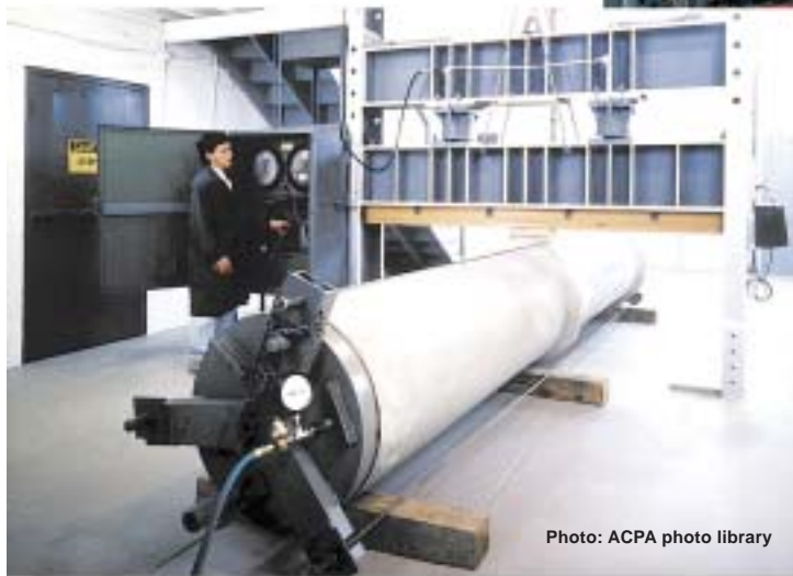
Concrete sewer and culvert pipes are designed to meet a specific cracking load.
