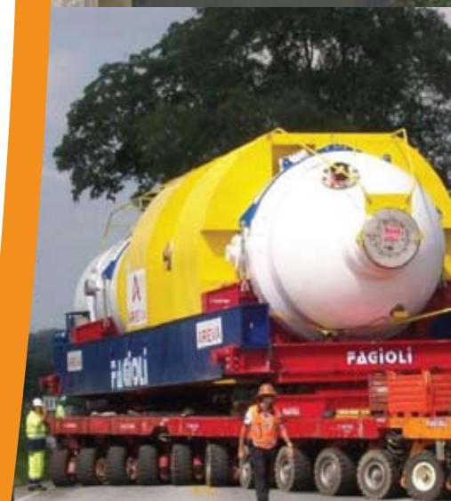
825 ton transport vehicles (26 axles and 208 wheels) and some the 100+ people that it took to make sure the move went off without a hitch.
