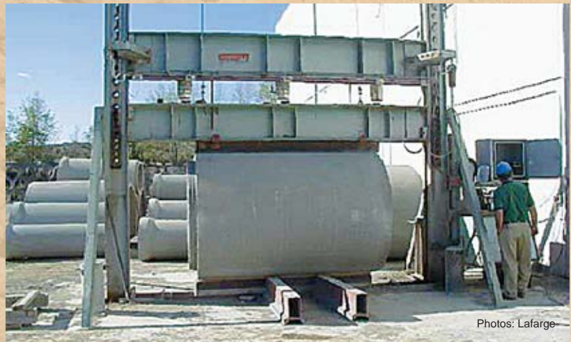
Technology for 21st century quality assurance. Testing of the strength of concrete pipe.
