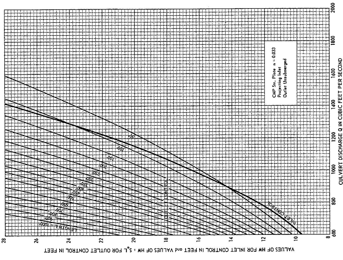
Interpolate for intermediate culvert lengths
