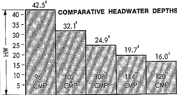
The geometric shape of the socket end of a concrete culvert pipe provides a more efficient entrance than the sharp edge of a corrugated metal pipe with or without a headwall. In addition, the relative smoothness of concrete pipe enables it to maintain equivalent discharge capacity at lower headwater depths than can be maintained by corrugated metal pipe.
