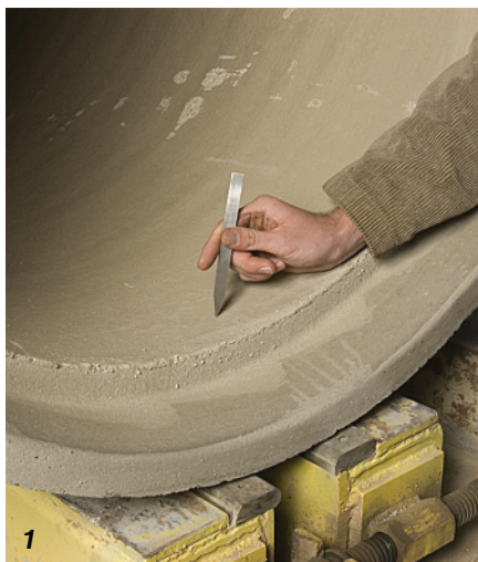
Pictures 1, 2, and 3 shown as if viewing the crack standing, kneeling, or through a video inspection, respectively.
