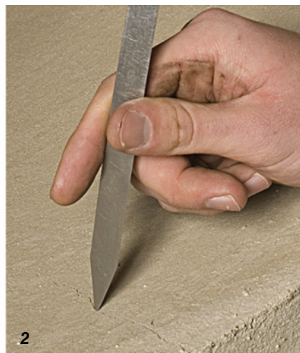
0.01-Inch Crack Measured in a 36-Inch, Class IV Pipe.
