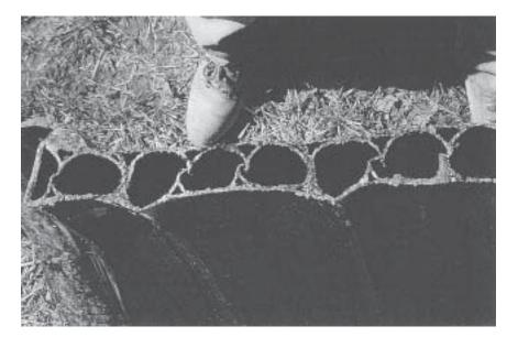
Obviously, the pipe wall profile was a key issue in this case. There are a variety of profile configurations available in HDPE drainage pipe, but little if any long-term testing has been performed on these products. While a method for evaluating the wall profile has been incorporated into the AASHTO design code since this pipe was installed, there still does not exist a requirement in M 294 to verify the profile dimensions. Should a designer use unverified properties in their design?
