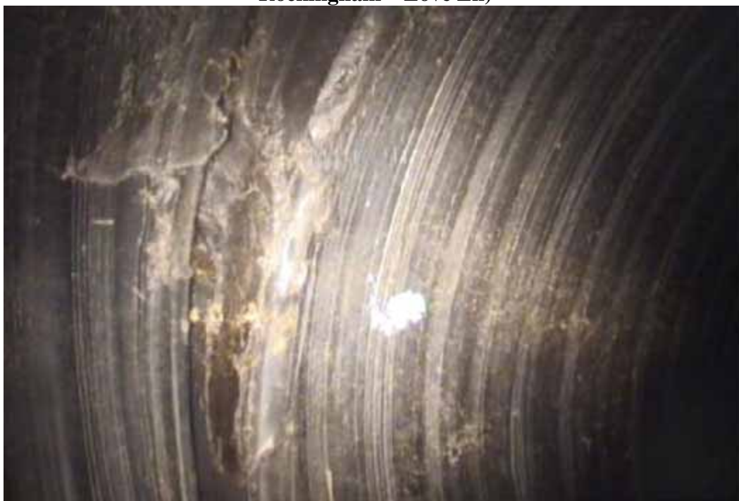
Figure 98 View of major joint displacement failure for pipeline No. 11 (Site No. 6: Rockingham – Love Ln)
