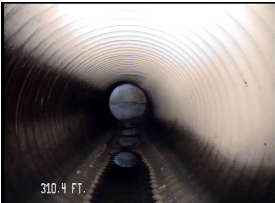
Figure 560 View of corrugation growth failure for pipeline No. 11 (Site No. 2: Apopka)
