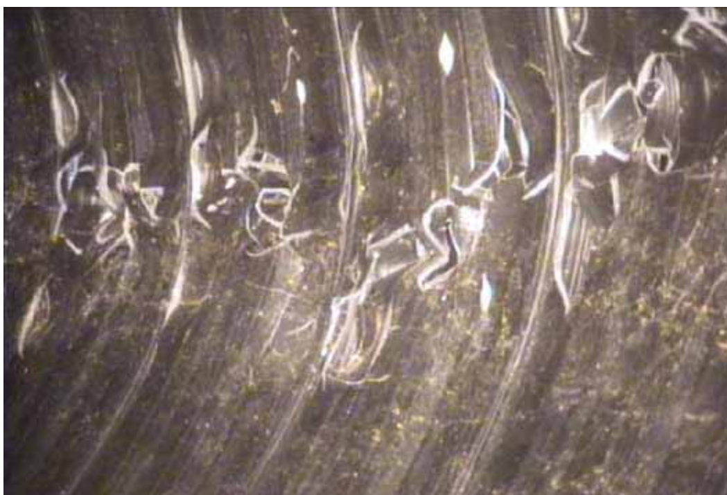
Figure 103 View of buckling and cracking failures for pipeline No. 11 (Site No. 6: Rockingham – Love Ln)
