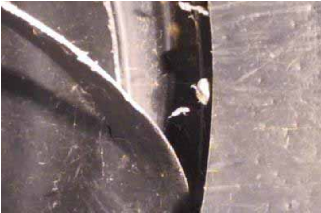
Figure 255 Cracking/fracture failure for Pipeline No. 1 (Site No. 1: Route 101)
