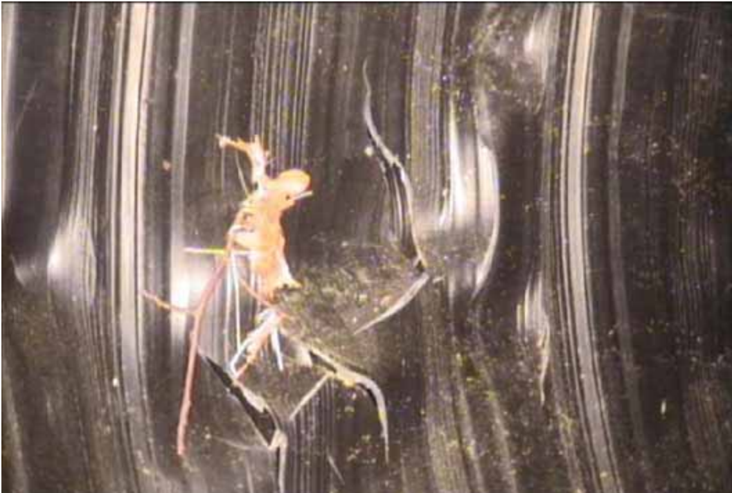
Figure 87 View of cracking failure for pipeline No. 10 (Site No. 6: Rockingham – Love Ln)
