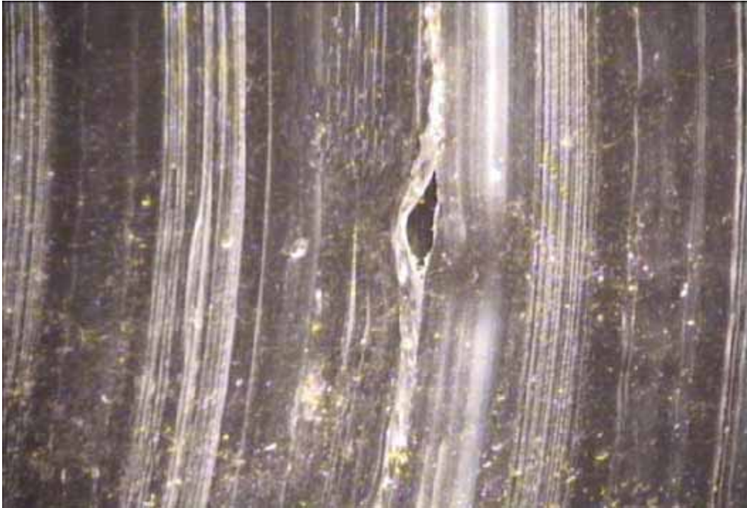
Figure 100 View of cracking failure for pipeline No. 11 (Site No. 6: Rockingham – Love Ln)
