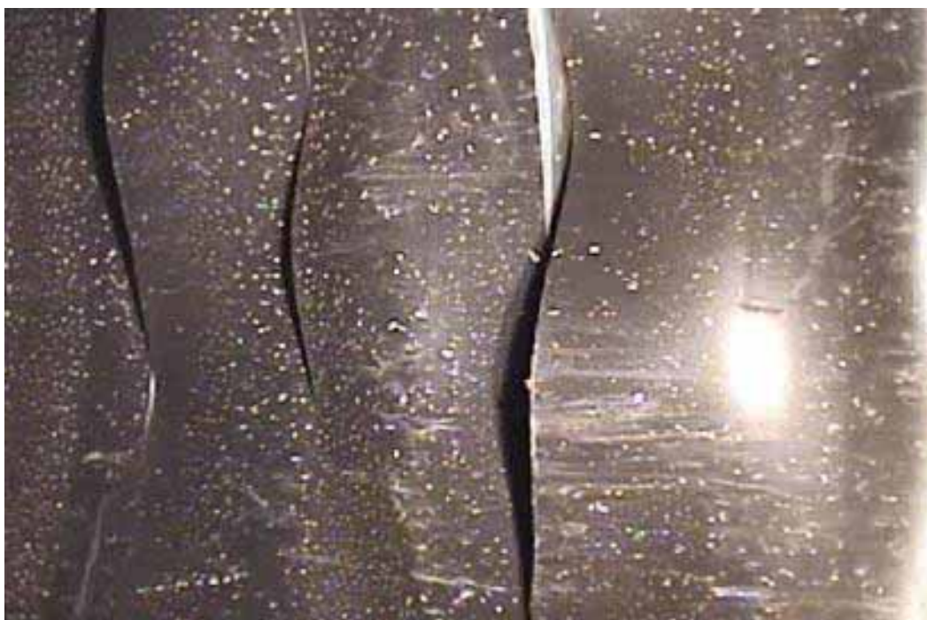
Figure 382 Cracking/fracture failure for Pipeline No. 9 (Site No. 2: Silver Creek Parkway)
