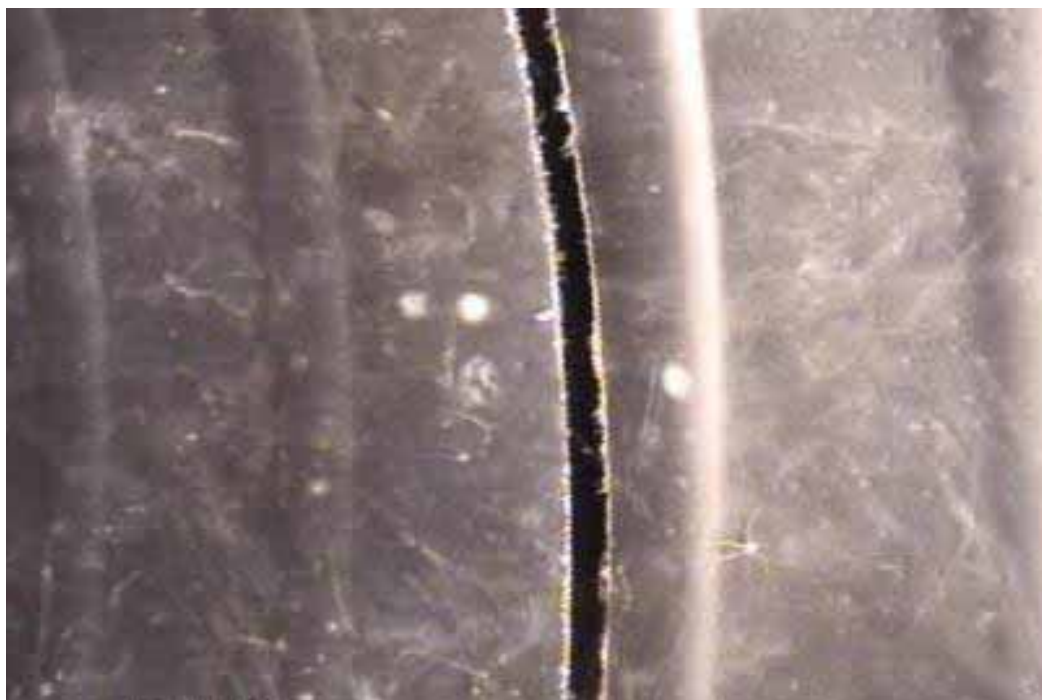
Figure 290 Cracking/fracture failure for Pipeline No. 7 (Site No. 1: Route 101)
