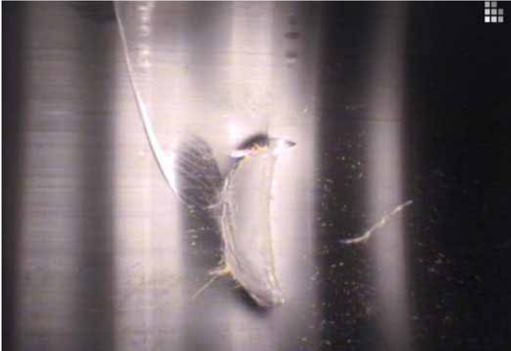
Figure 182 View of cracking/fracture failure for pipeline No. 19 (Site No. 6: Brooklyn Park - DuPont)
