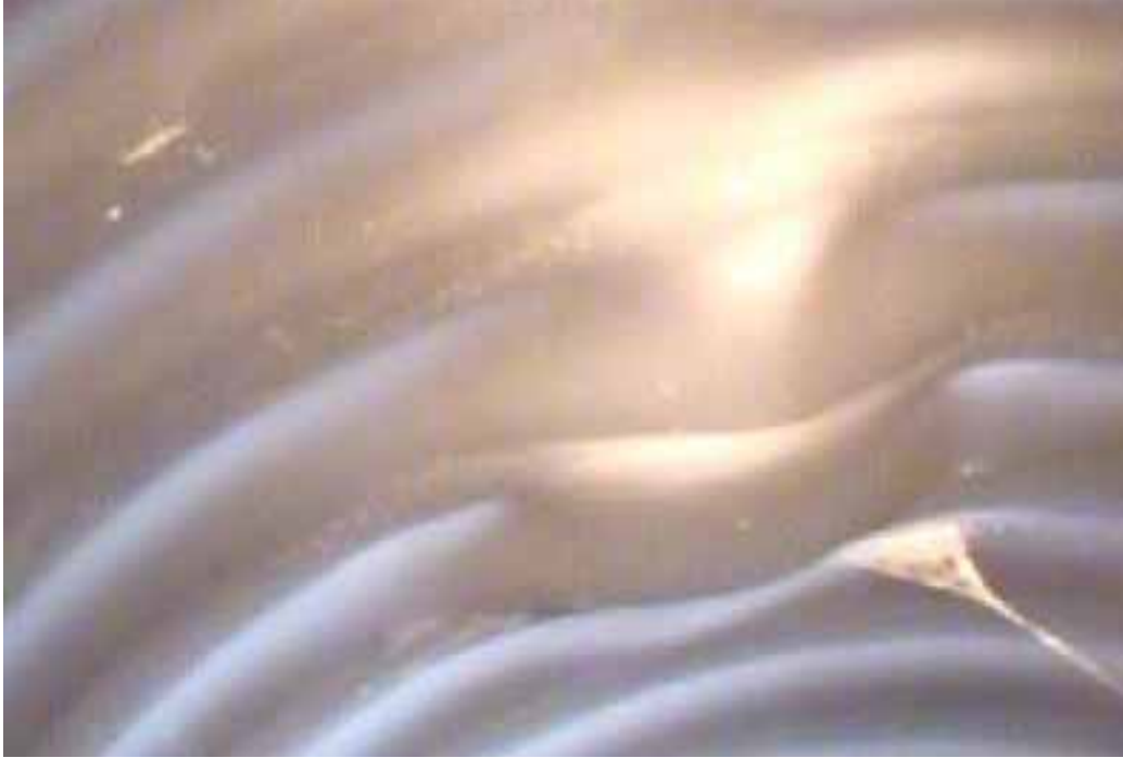
Figure 372 Cracking/fracture, corrugation growth, and inverse curvature failure for Pipeline No. 6 (Site No. 1: Legacy Parkway)
