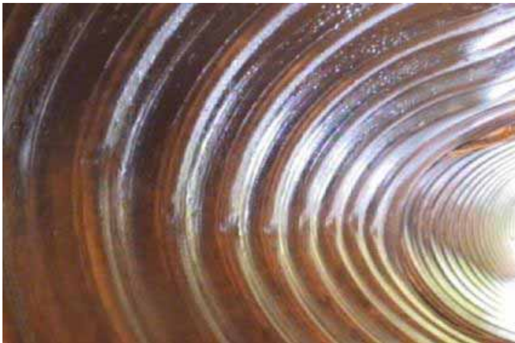
Figure 421 Corrugation growth, excessive deformation, and buckling failure for Pipeline No. 8 (Site No. 7: West Island Road)
