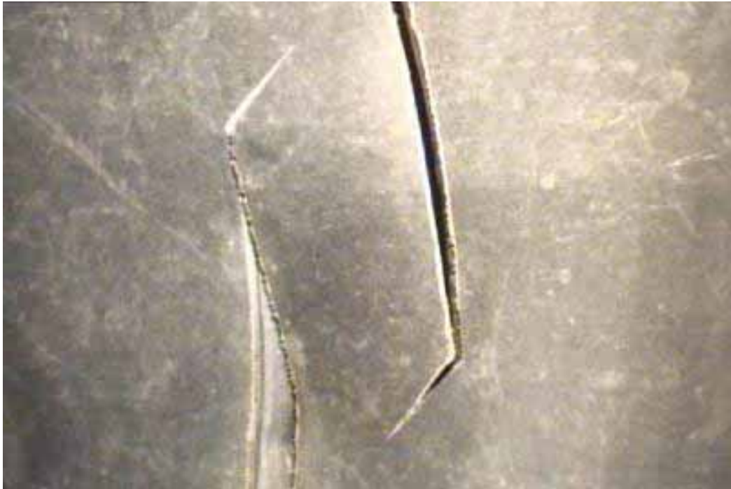
Figure 276 Cracking/fracture failure for Pipeline No. 4 (Site No. 1: Route 101)
