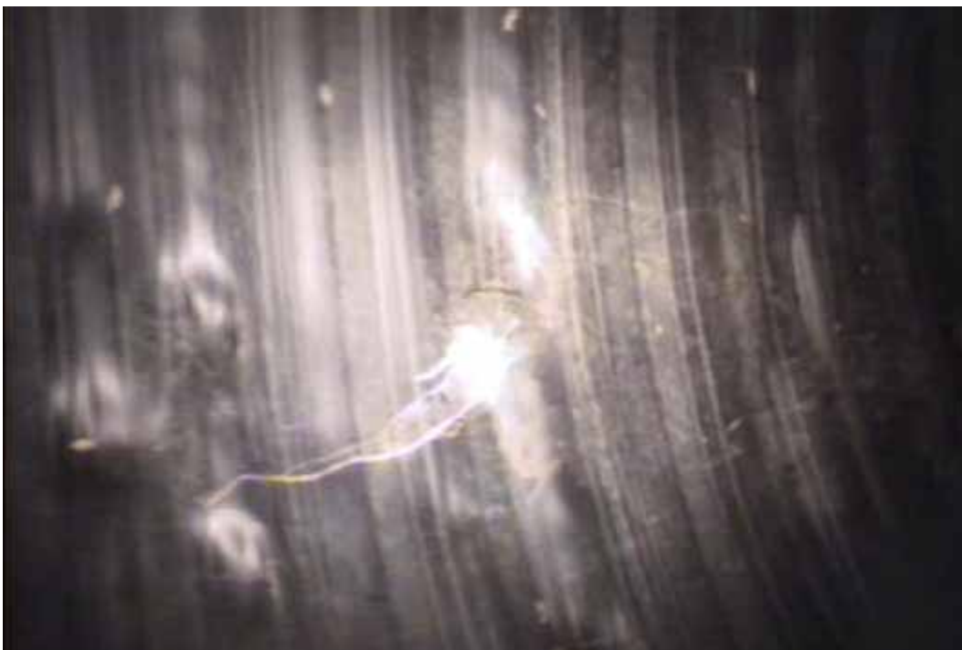
Figure 105 View of cracking failures for pipeline No. 11 (Site No. 6: Rockingham – Love Ln)
