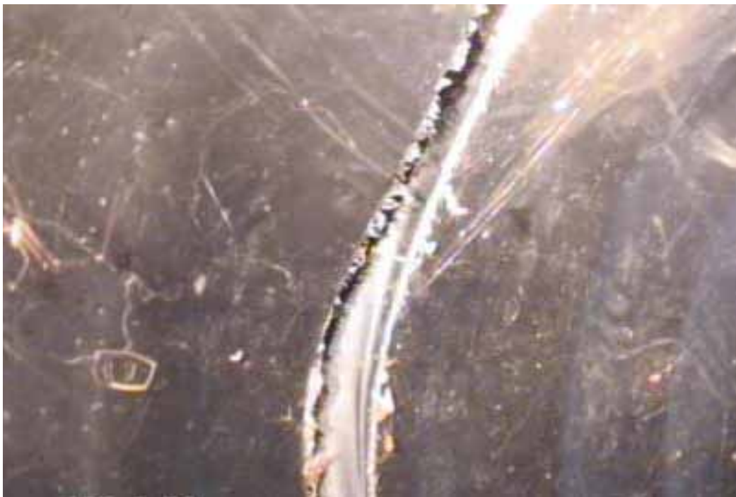
Figure 312 Cracking/fracture failure for Pipeline No. 10 (Site No. 1: Route 101)
