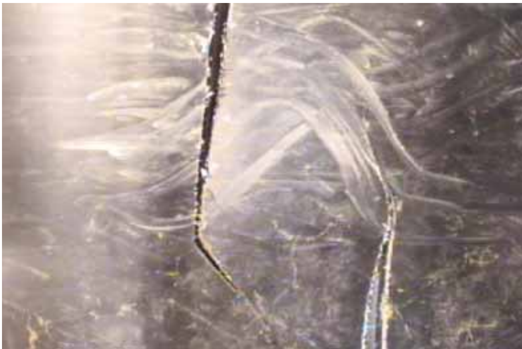
Figure 280 Cracking/fracture failure for Pipeline No. 5 (Site No. 1: Route 101)
