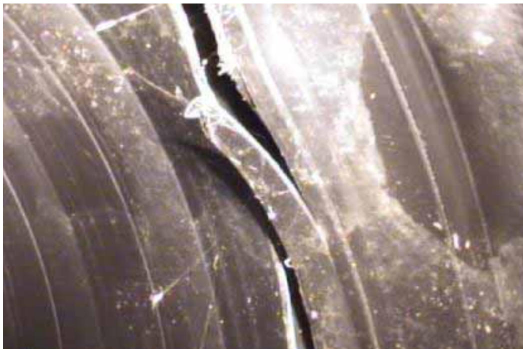
Figure 414 Cracking/fracture and inverse curvature failure for Pipeline No. 6b (Site No. 6: Houghton County M92)
