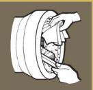
Carefully clean all dirt and foreign substances from the joining surfaces of the bell or groove end of pipe.
