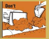
Backfill material should be readily compactible and job excavated material and should not contain large stones, boulders, frozen lumps or other objectionable material. Backfill should be placed and compacted in layers as specified.
