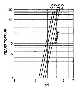
Figure 1: Concrete Pipe Culvert Life
