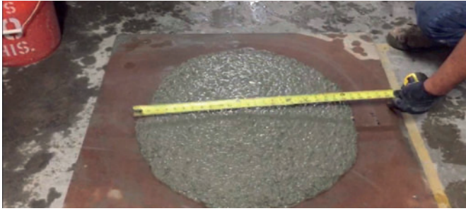
Slump flow test
