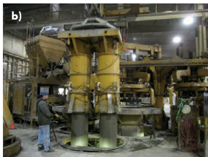
Figure 2. Manufacturing equipment: (a) Packerhead production; (b) Hawkeye production.
