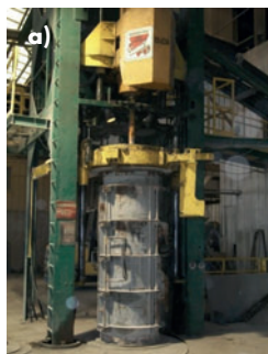
Figure 2. Manufacturing equipment: (a) Packerhead production; (b) Hawkeye production.
