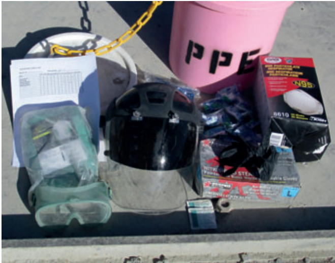
A five gallon, high visibility bucket with several personal protective equipment eliminates the barrier to use it
