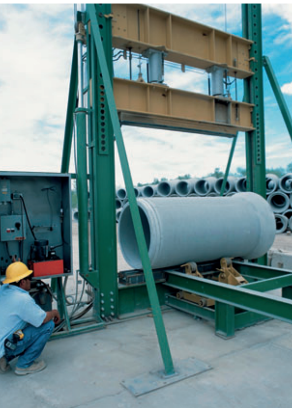
Three-edge Bearing Test. Photo: Courtesy American Concrete Pipe Association
